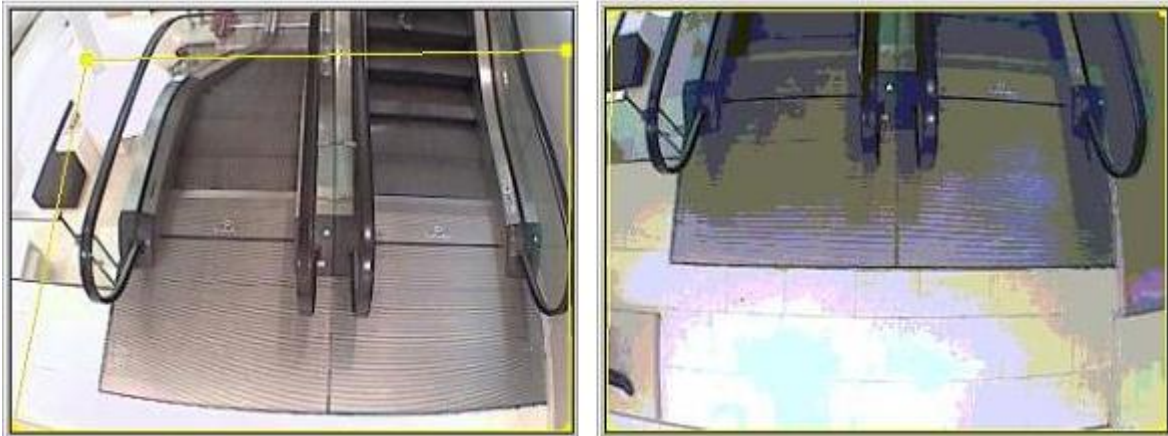
Figure 5: A bad (left) and a good (right) camera view of an escalator
