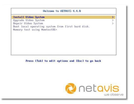
Menu items with an ">" open a new submenu, while the other items directly start the desired operation. Press **ENTER** to start an operation or open a submenu and pressing **ESC**to go back to the previous menu. The install submenu looks:
